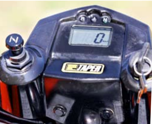
ABOVE: Its instruments are basic by today's standards. It's not often you see a choke anymore, but that's because this HO engine has a carb, not EFI.
